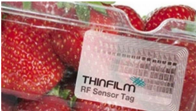
Figure 2: Radio Frequency Sensor Tag for food chain and quality control 6
